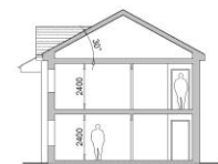
Proposed Section A-A'
